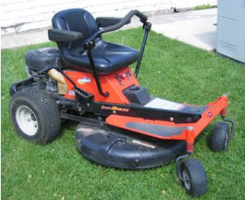
It took a little trial and error, getting used to 'steering' it using those levers instead of a conventional steering wheel. It will turn in an abrupt circle where it stands! Gotta be careful or one could become dizzy:o)
